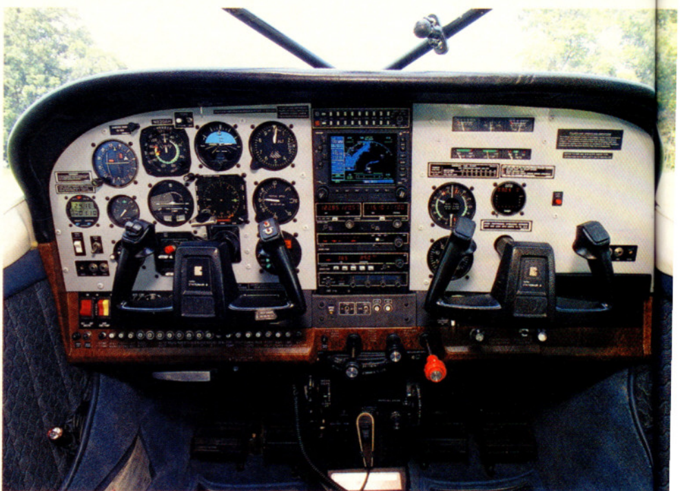
Clockwise from top left: Wipaire’s copilot door is a huge convenience for the seaplane pilot and doubles as an emergency exit. The Landing Gear Advisory System is included with a new set of Wipaire floats. The emergency gear extension lever and the water control lever are installed between the front seats. The instrument panel is outfitted with a Garmin GNS 530, Sandel electronic horizontal situation indicator (EHSI), and an S-Tec System 60-2 autopilot with GPSS.
